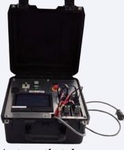
Automatic take-up device controller The cable is automatically wound and unwound according to the altitude of the drone.
