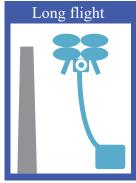
When flying vertically, such as when checking high places, the cable will not get caught and you can fly for a long time.
